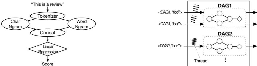
(a) A DAG for sentimental analysis from text inputs consisting of operators for featurization (ellipses), followed by a ML model (diamond). (b) Each DAG is compiled as a chain of virtual function calls. When a prediction request is issued, a thread is dispatched to execute the chain as a single (black box) function call.
