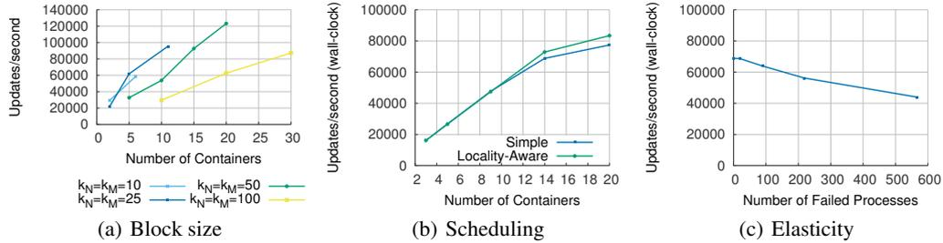
Figure 2: We test the performance of our system across a variety of settings. (a) We observe that larger blocks are faster to process but smaller blocks offer more parallelism. (b) We observe that both scheduling algorithms scale linearly to additional containers, with the locality-aware scheduler being able to more efficiently use higher numbers of containers. (c) Our system is highly fault tolerant, with many container failures causing only a slight decrease in performance.
